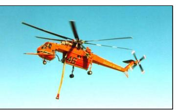
The tank is fitted with a fast self-fill snorkel that allows it to hover-fill from a variety of water sources. The microprocessor controlled tank system is capable of delivering multiple drops. In addition the *Air-crane* is fitted with the Sea Snorkel. The Sea Snorkel allows the *Air-crane* to fill from salt-water sources during forward flight.
