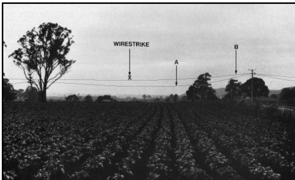
Figure 19. Focussing on high and low wires together can create the illusion that the higher wire (B) is further away than the lower wire (A)
