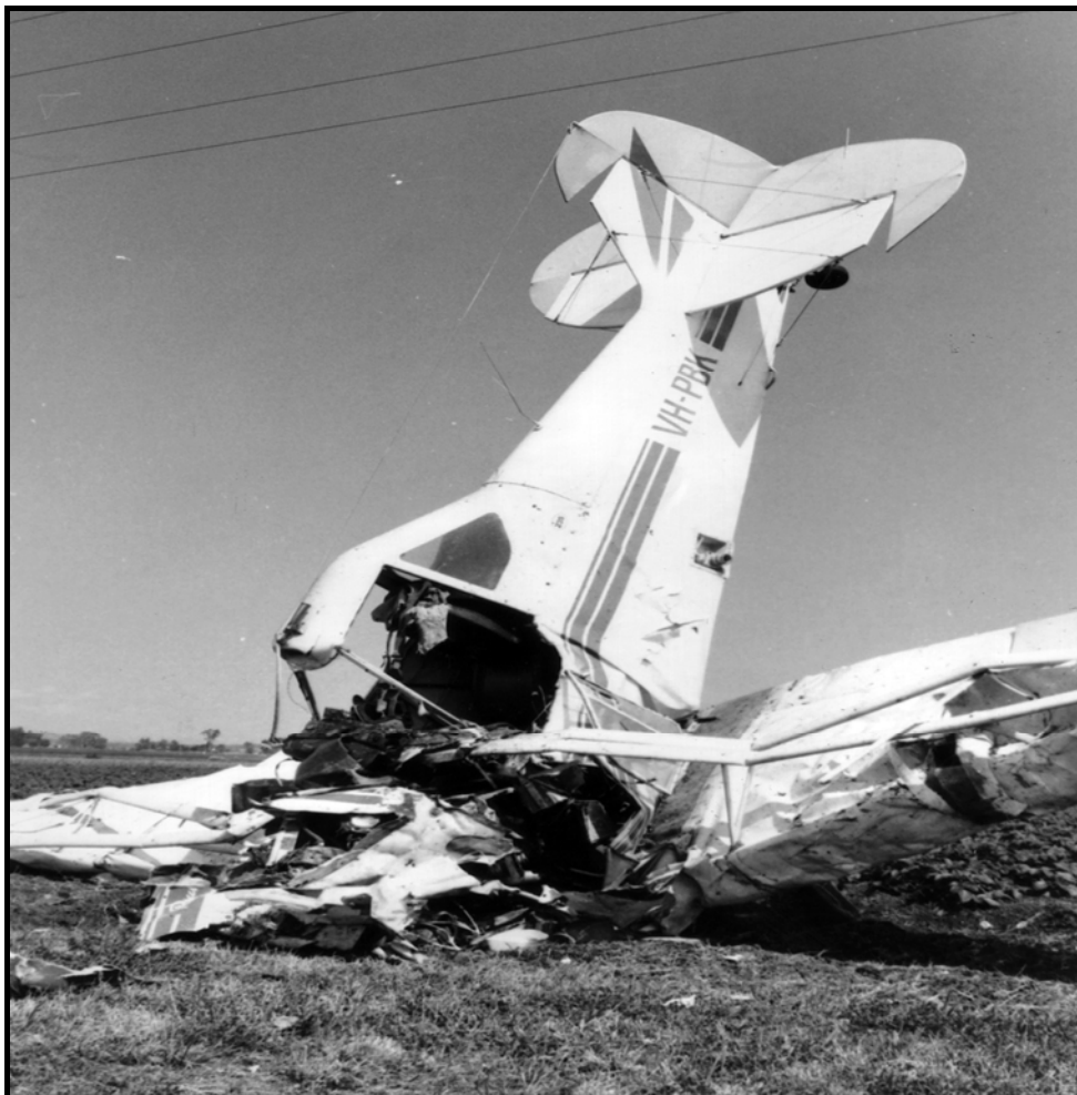
Figure 21. Aircraft after striking a high tension powerline during a pull-up manoeuvre
