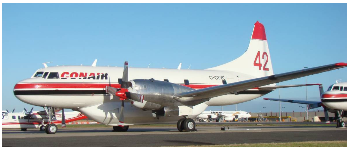
Conair Convair CV-580 with RADS II-220 retardant delivery system.
