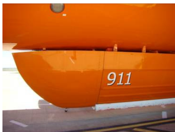
Forward fairing tank and No. 1 Tank
