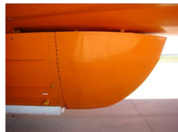
Aft fairing tank and No. 3 Tank.
