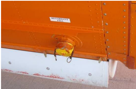
Standard filling port 3" camlock male fitting.
