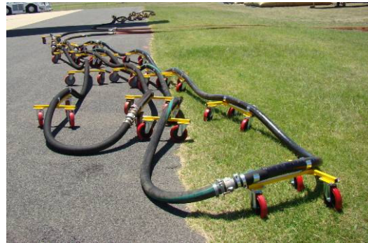
3 X 25 metre loading hoses and ramp skates.
