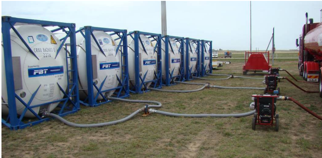
Series of portable 30,000 litre ISO-containers
