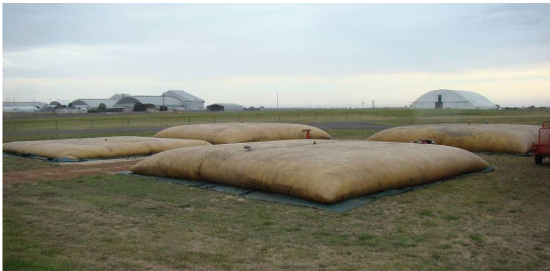
Bladder Farm shows 4 portable inflatable containers.
